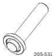
Halfshaft oil seal installer 205-532
