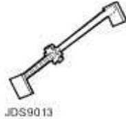
Brake pedal hold-down tool JDS 9013
