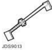
Brake pedal hold-down tool JDS 9013
