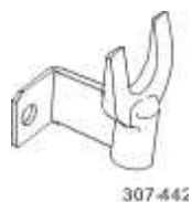
Halfshaft splitter 307-442
